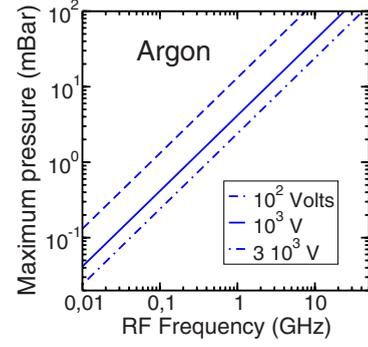
FIG. 2. (Color online) The maximum simulation pressures and different microwave peak amplitudes  $V_o$  for argon with  $N_s = 200$ .
