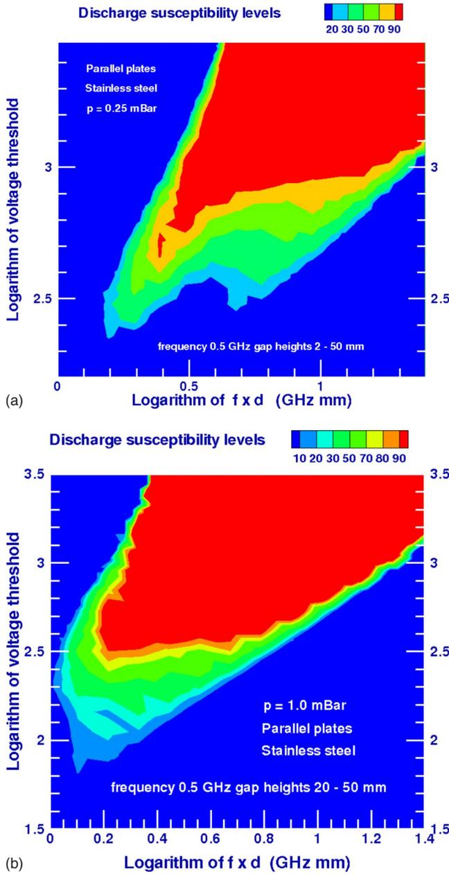
FIG. 7. (Color online) The rf voltage thresholds for rf breakdown as a function of  $f_w D$  for large values of the ratio  $v_m/f_w$ . The decimal logarithm is employed in both axes.
