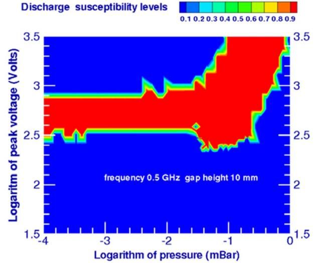
FIG. 4. (Color online) The predicted rf breakdown voltage thresholds corresponding to the experiments of Ref. [17] for different gas pressures. The decimal logarithm is used in both axes.
