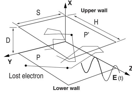
FIG. 1. The model geometry with the lower ( $P$ ) and upper ( $P'$ ) coated surfaces separated by the gap height  $D$ .
