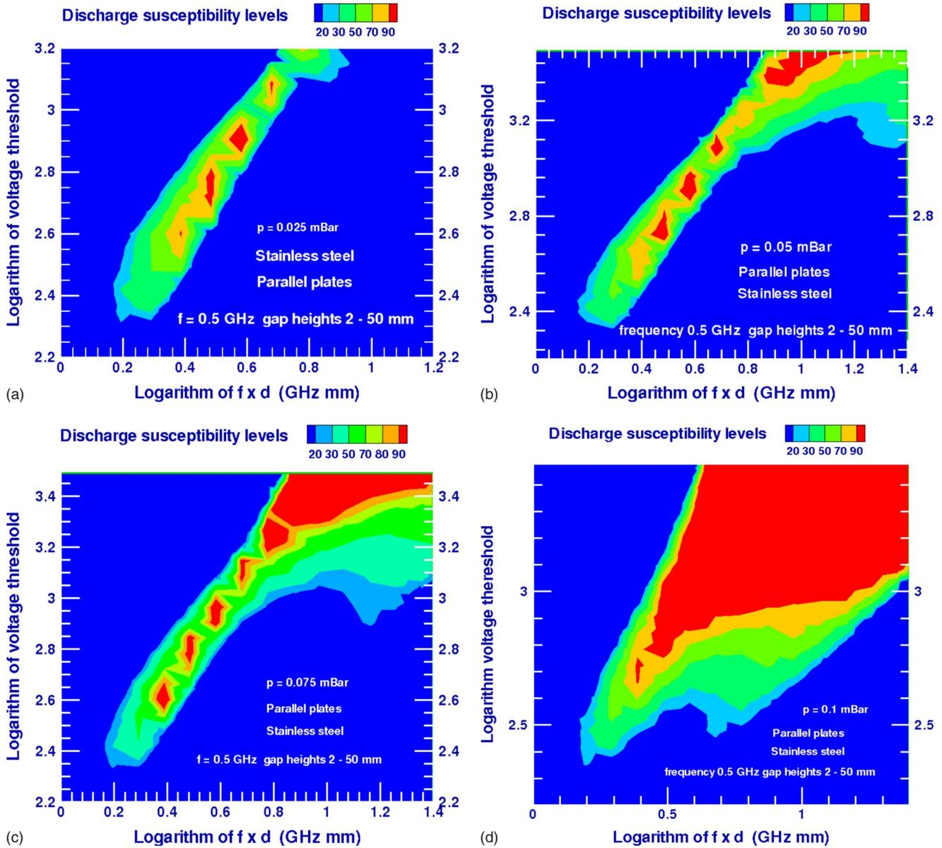
FIG. 6. (Color online) The rf voltage thresholds for rf breakdown in argon as a function of  $f_w D$  for different values of the ratio  $v_m/f_w$  within the collisional multipactor plasma range of pressures. The decimal logarithm is employed in all axes.
